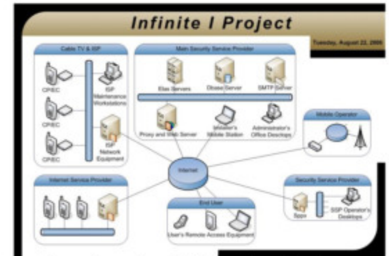
Security system (Infinity-I) architecture
