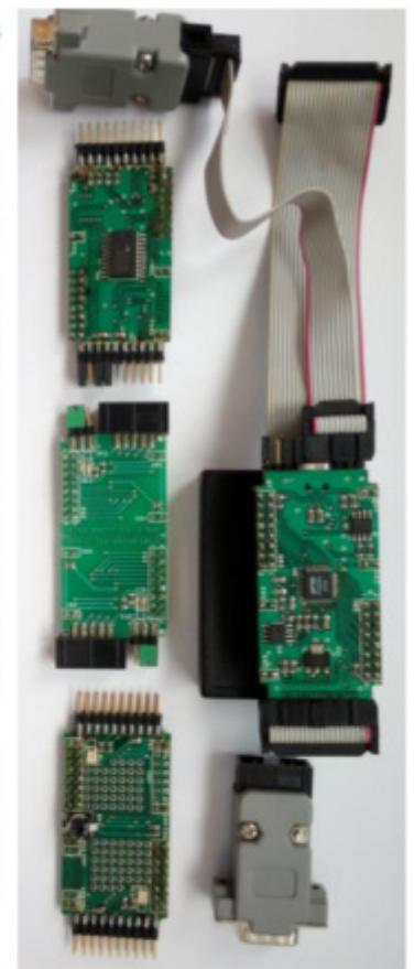
MultiFDS: FTDI FT2232 based TTL Serial/RS232/JTAG adapter (2007)
