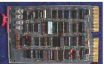
Punch tape subsystem for LSI-1123 I/O
